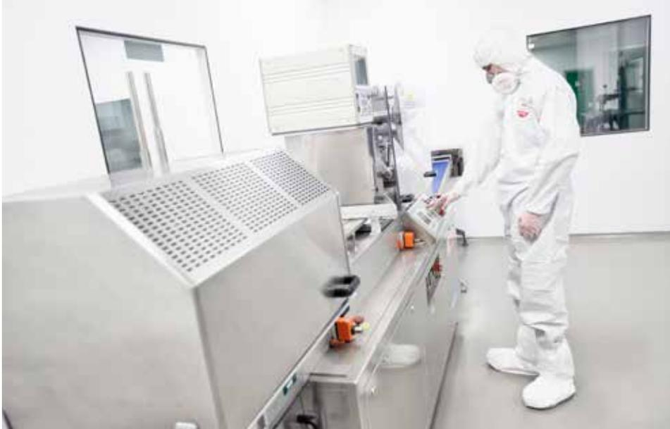
*Millmount introduced a new high containment blister packaging line geared for high-speed quick changeovers using a standard blister size*
